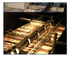
Testing in accordance with the standard IEC 61914:2009 clause 6.4.3, a current of 106KA was applied to the cable. An inspection of the test object then confirmed that there had been no damage to either the couplers or the tray with both appearing to be in the same state as prior to the tests taking place. In line with clause 6.4.4 another current of 106KA was again passed through the same test object. with an inspection once more confirming that there had beenno damage to the system.
