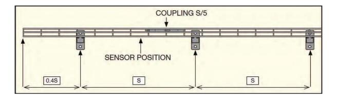
Note: The maximum deflection of 1/100 is always reached for a lesser load than that of the safety load. (The breaking point divided by a safety co-efficient of 1.7). CEI/61537
